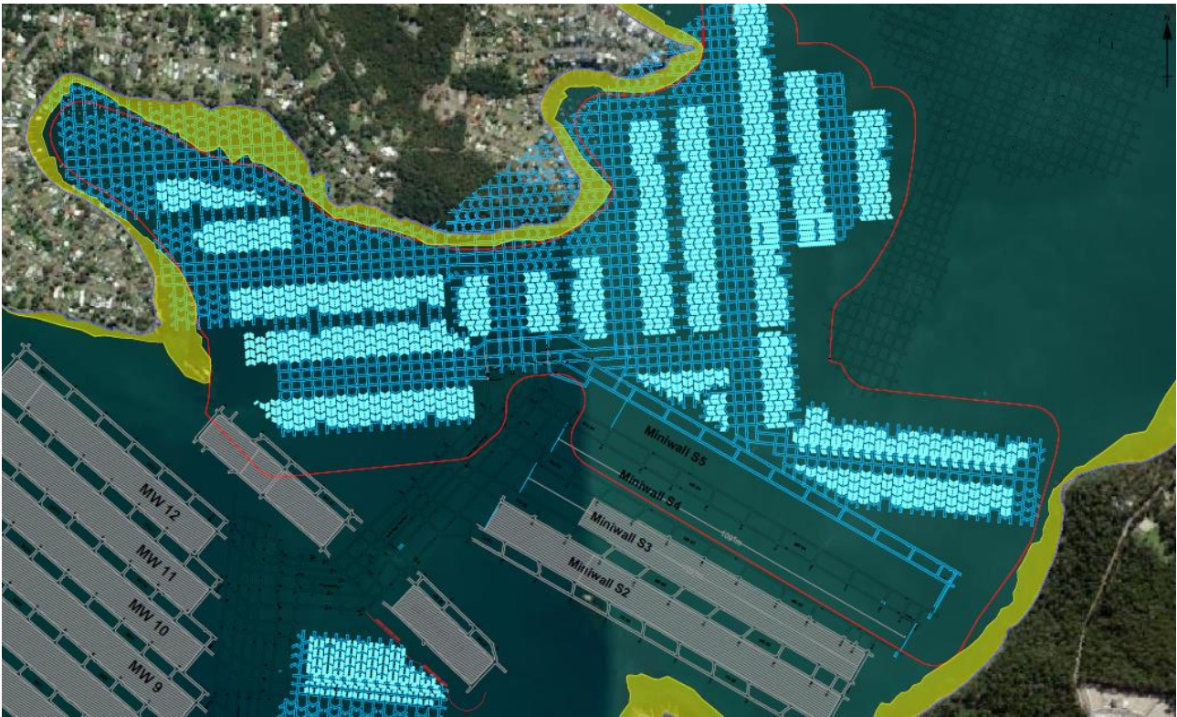
Figure 2 - Predicted Subsidence impact areas due to extraction methods under Lake Macquarie (Hill, 2020)
